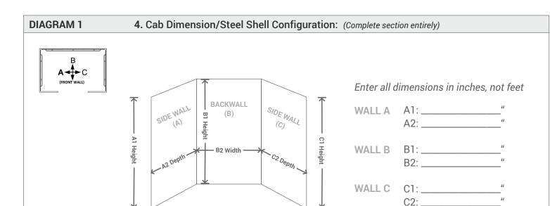
\*Height is measured from floor to canopy (not ceiling) \*If cab has cove/obstruction, measure height from floor to bottom of the cove/obstruction
